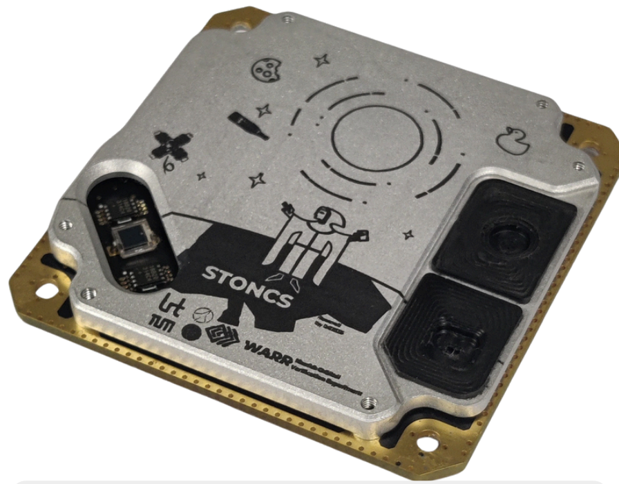
Figure 1: STONCS PCB with the shield and apertures installed
